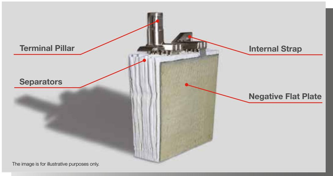
FIAMM FLB RANGE USE AGM (ABSORBED GLASS MAT) TECHNOLOGY. THE ELECTROLYTE IS ABSORBED IN FIBERGLASS SEPARATORS WITH 99% INTERNAL GAS RECOMBINATION EFFICIENCY. BLOCS ARE GRANTS NON-SPILLABLE AND MAINTENANCE FREE THEREFORE REQUIRES NO TOPPING UP OF ELECTROLYTE DURING ITS WHOLE LIFE. LOW SELF-DISCHARGE ALLOWS 6 MONTHS SHELF LIFE.
